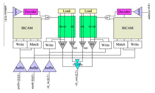
Fig. 9. The BCAM architecture for the high-speed IPv6 routing lookup system.
