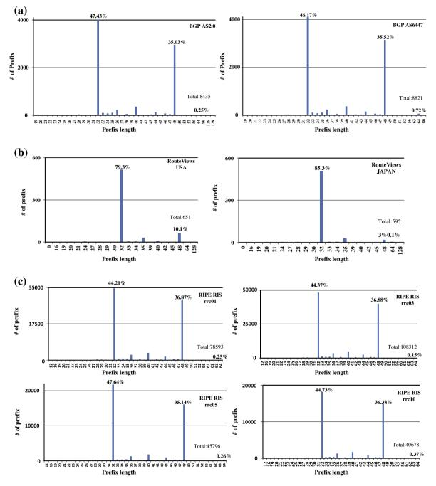
Fig. 2. Prefix length distribution: (a) the IPv6 BGP table; (b) the Route Views project; and (c) RIPE RIS project.
