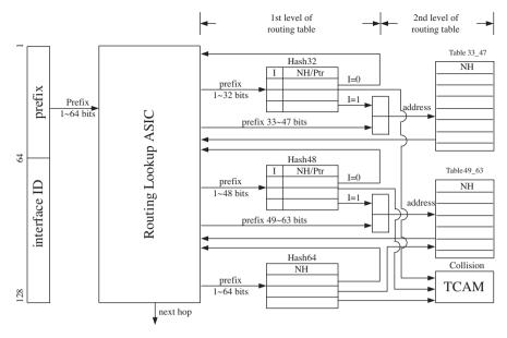
Fig. 4. The architecture of routing lookup system.
