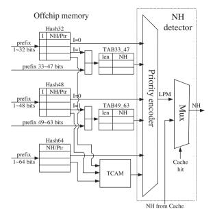
Fig. 11. The architecture of the NH detector.
