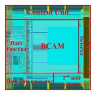
Fig. 13. ASIC layout of the routing lookup system.
