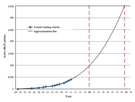
Fig. 6. IPv4 routing table size with estimated approximation line.
